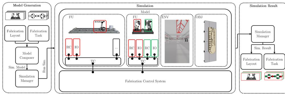
Figure 3. Simulation Workflow
